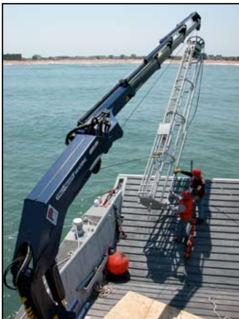
R/V Pelican deploying vibracore
